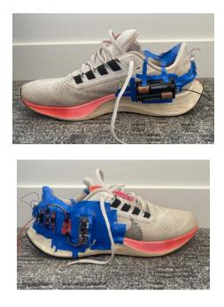
The above figure shows the design of the actual prototype. The hardware was connected to a Nike Pegasus 38 running shoe. Cardboard was placed below the hardware components for stability; the unit was secured to the show via duct tape.
